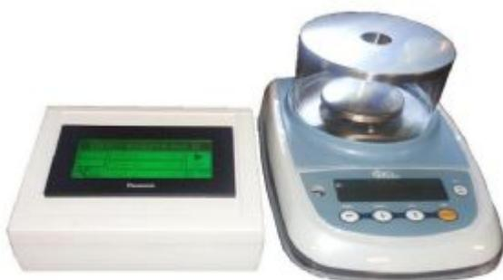
Equipped with a precision scale, in the full version, CC10 can do analyses both for the determination of yarn count according to National and International Yarn Count systems and the GSM of fabrics, paper, plastic and other materials.
